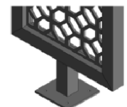
Welded square tube frame with pedestal mounts
