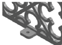
Welded on angle tabs
