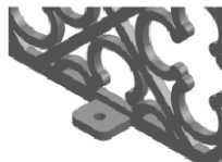
Welded on angle tabs
