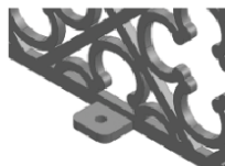
Welded on angle tabs
