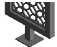
Welded square tube frame with pedestal mounts
