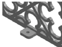
Welded on angle tabs
