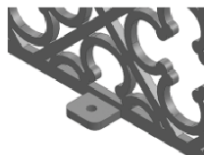
Welded on angle tabs
