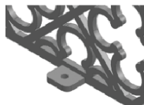
Welded on angle tabs
