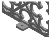
Welded on angle tabs
