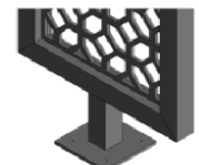
Welded square tube frame with pedestal mounts
