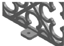
Welded on angle tabs
