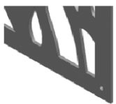
1/4" mounting holes around edge of panel
