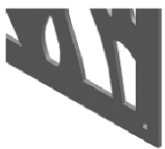
1/4" mounting holes around edge of panel
