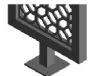
Welded square tube frame with pedestal mounts
