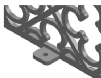
Welded on angle tabs
