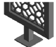
Welded square tube frame with pedestal mounts
