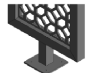
Welded square tube frame with pedestal mounts
