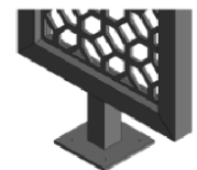
Welded square tube frame with pedestal mounts
